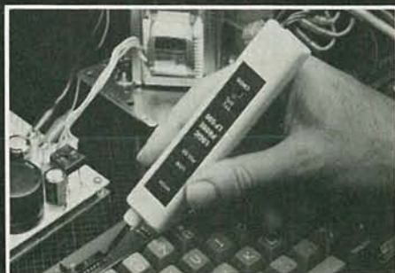
After you build this digital logic probe, you'll explore the operation of the Sanyo detached "Intelligent" keyboard and its dedicated microprocessor.
