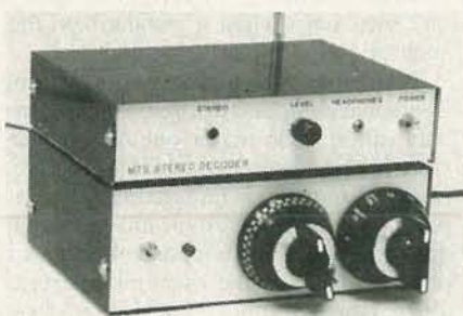
AN OUTBOARD TUNER lets you use the circuit with a TV that lacks audio outputs. Next time, we'll see many other ways of using the circuit.
