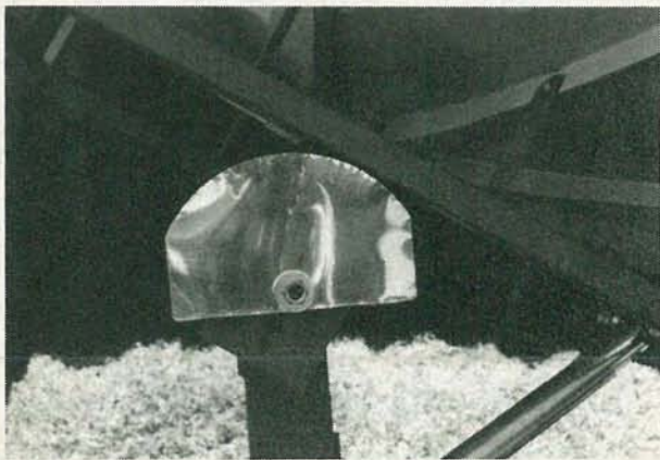
FIG. 3—AN ALUMINUM COOKIE SHEET is used as a dial. The antenna mount rotates about a fixed dial with a scribed line on the frame as an index.
